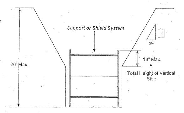
All excavations 20 feet or less in depth which have vertically sided lower portions that are supported or shielded shall have a maximum allowable slope of 3/4: 1. The support or shield system must extend at least 18 inches above the top of the vertical side.
