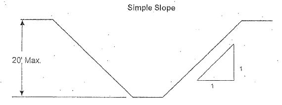
All simple slope excavations 20 feet or less in depth shall have a maximum allowable slope of 1; 1
